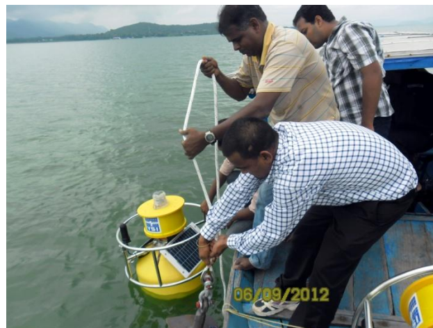
Water quality monitoring buoys are deployed throughout Chilika Lake and transmit data to scientists working to conserve the lake ecosystem.
